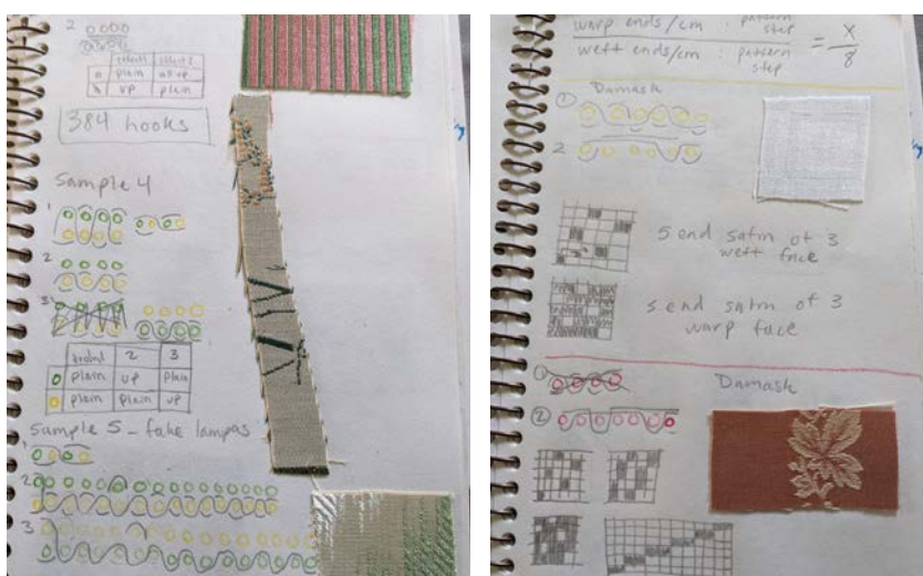
Top: A series of punch cards is mounted on the loom to create the pattern. Middle: Jacquard draft preparation includes color-coding the different weave structures on paper, counting warp and weft floats, and removing any long floats. Bottom: During her Jacquard studies, Yvonne made comprehensive planning and interlacement notes.
