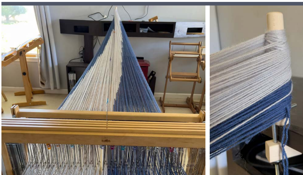
Left: The completed warp for Shawl 1 is ready to wind on to the loom. Notice the warping guide string with clips attached and the clips on Shaft 4 that indicate threading repeats. Right: The warp for Shawl 1 wrapped on the peg. Each end is wrapped an extra time around the peg to maintain even tension and so the join position doesn't slip.
