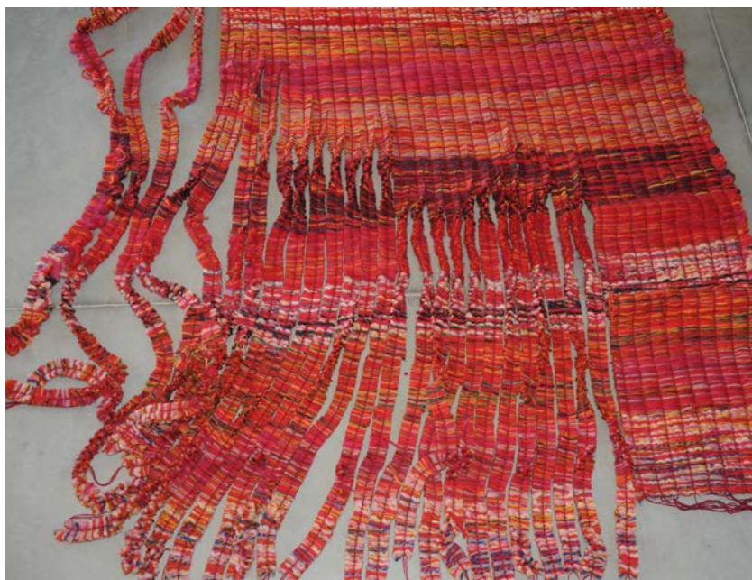
Top: Catherine's first warp is an extreme example of crammed and spaced. Eight ends, sett tightly, are spaced about an inch apart. The crammed ends hold the weft firmly in place while the spaces allow ample room to cut the fabric into chenille yarn. Bottom: After weaving the fabric, Catherine carefully cuts between the warp threads to create a chenille yarn.
